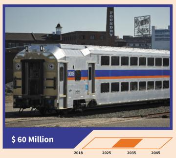
The MARC IV railcars are the newest railcars in the fleet. These railcars are scheduled for a midlife overhaul in 2028. The overhaul will include the replacement of major component parts, electrical systems, seats and other elements that ensure a safe and pleasant ride for passengers.
