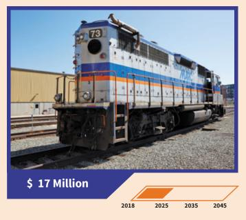
Entered into service in 1987 and were last overhauled in 1998. The GP39H-2 locomotive is the oldest locomotive in service in the MARC fleet. To keep these six locomotives operating reliably and to extend their useful life, MDOT MTA will overhaul the locomotives by replacing key components. The GP39H-2 locomotives will be removed from service in pairs to undergo the mid-life overhaul.
