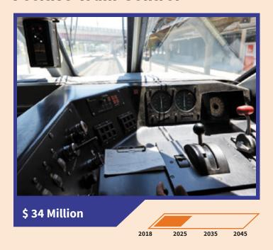
Positive Train Control (PTC) is technology used on railroads to minimize and prevent trains from colliding with one another due to human error.
