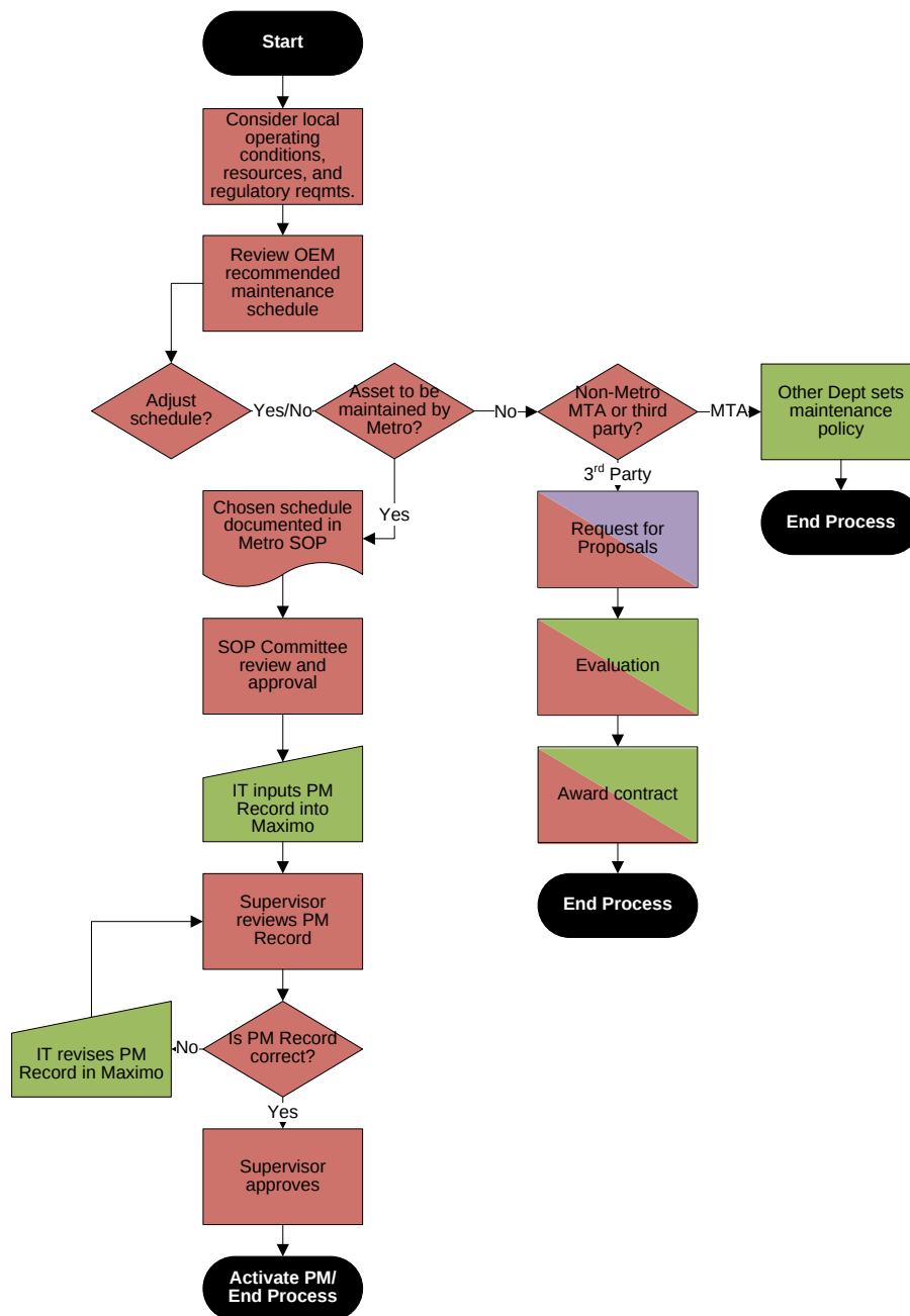
Figure 9.2- Metro's maintenance policy process.
